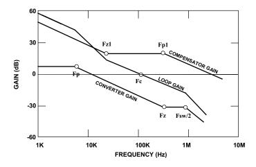
Figure 8 — Bode plots for voltage loop design
