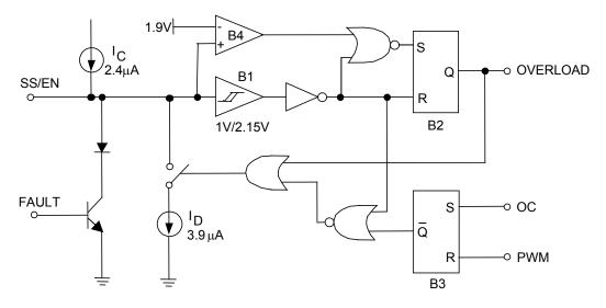
Figure 3 — Soft-start and Overload Hiccup Control Circuit
