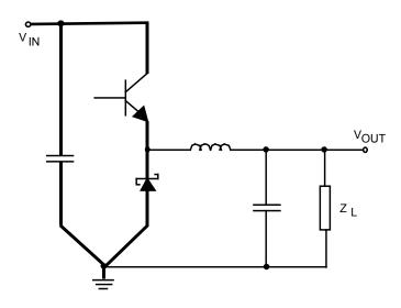
Figure 9 — Pulse current Loop
