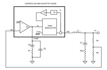
Figure 7. Block diagram of control loops
