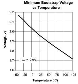
Figure 5 — Typical Minimum Bootstrap Voltage required to Saturate Transistor (I<sub>SW</sub>= -2.6A)
