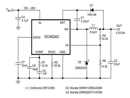
Figure 11. 700kHz 10V-26V to 3.3V/2A Step-down Converter
