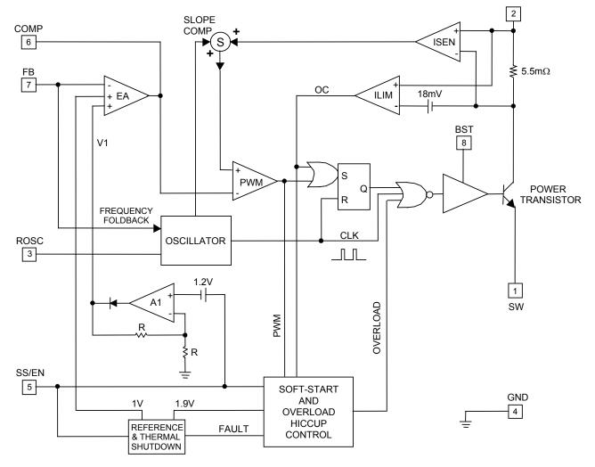
Figure 2 — SC4524C Block Diagram
