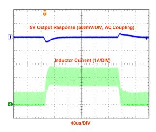
Load Transient Response (I<sub>o</sub>= 0.3A to 2A)
