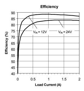
Figure 1. 1MHz 10V-28V to 5V/2A Step-down Converter
